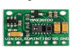
Fig 2 Heart Beat and Pulse Oximeter Sensor
